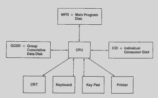
Fig. 1. A schematic diagram of the interrelationships between the Central Processing Unit (CPU), the disk drives for each major function and the input/output devices. The CRT (Cathode Ray Tube) or VDU (Video Display Unit) is actively used during data input, review and editing while the printer is used primarily for final reporting.
